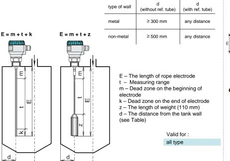
For correct measurement it is important to avoid installation in the high extended type tank connections
